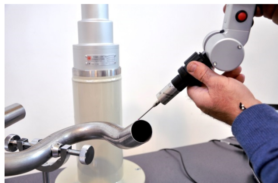
Pipe measurement by laser fork and touch probe (LP2 Renishaw™)
