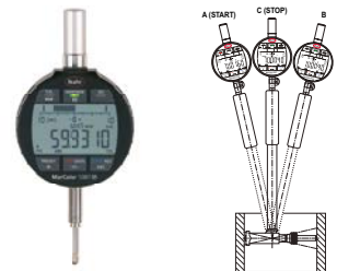
1087 BRi for dynamic comparative inner/outer measurements
